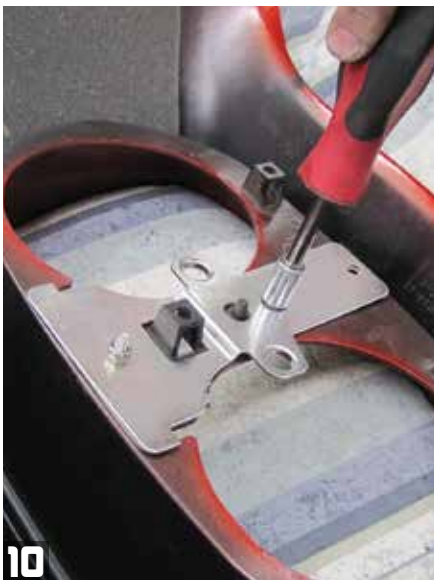
10 After threading on the two Cyron-supplied locknuts, tighten them using a 10mm socket.
