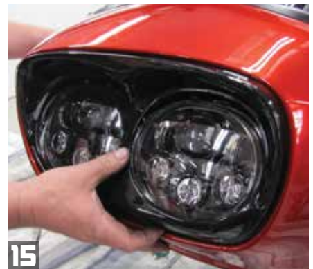
15 Insert the Cyron headlight bezel into the front of the fairing. Make sure the bezel's four clips fully seat and clip into their slots in the fairing.
