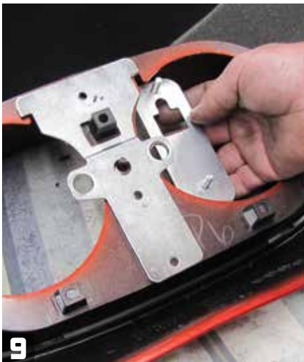
9 Insert the Cyron front support bracket into the other side of the fairing and slip its two studs through the holes you drilled in Step 7.
