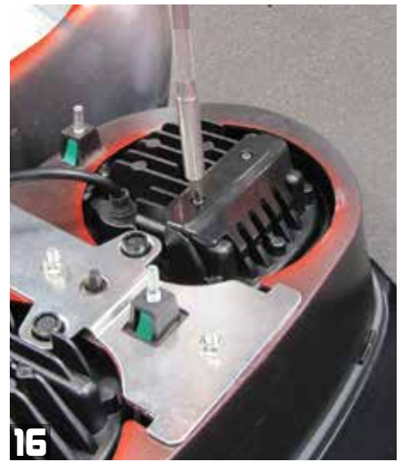
16 The Cyron wire harness protection bumper is secured to the left headlight using the two Cyron-supplied screws and a #2 Phillips screwdriver. Be sure to align the headlights once the fairing is reinstalled.
