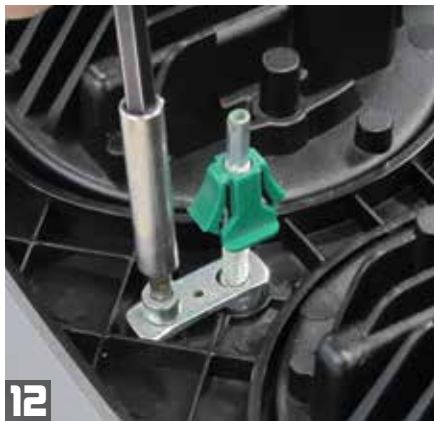
12 After threading the square plastic clips onto the round bolts so they match the position of the stock ones for each location on the stock headlight, install them onto the new Cyron headlight (balled end in round socket) using a 5/16" Allen.
