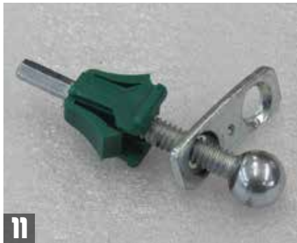
11 Slip a Cyron square washer onto each of the rounded bolts with the chamfered side facing the round ball on the bolt. Then thread on a square plastic clip onto each round bolt. Note: the center one is shorter than the other two.
