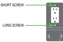
Install the long colored screw in the lower hole of the wall plate. Apply pressure on the plate as you start to install this screw, making sure the screw is lined up with both the outlet and the electrical box. Tighten the lower screw so the wall plate and the outlet are firmly in place. Turn on the fuse panel to restore electricity to the outlet.
